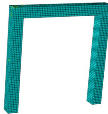
Figure 12. Meshing of the Reinforced Concrete Frame.
