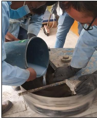
**Figure 1.** Pouring of the nano-silica mixture into the mix.
