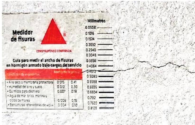
Figure 6. Crack Comparator Card
