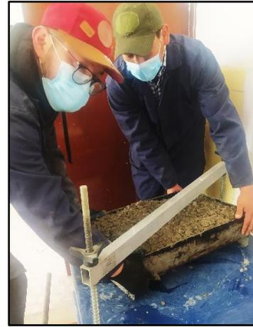
**Figure 2.** Placement of the mixture on the vibrating table for 10 seconds to achieve leveling and smoothing.
