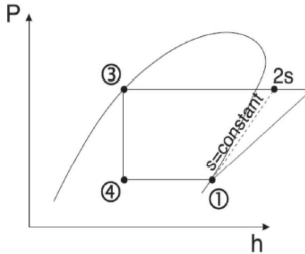
Fig. 2: P-h diagram of refrigeration cycle.
