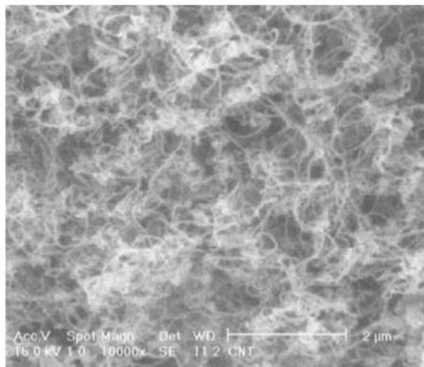
Fig. 3: Typical SEM image of carbon nanotubes.
