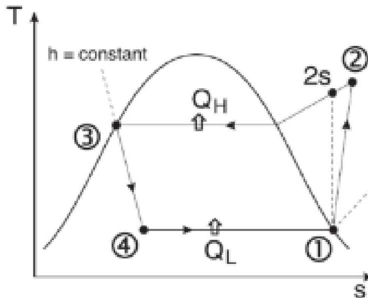
Fig. 1: T-s diagram of refrigeration cycle.
