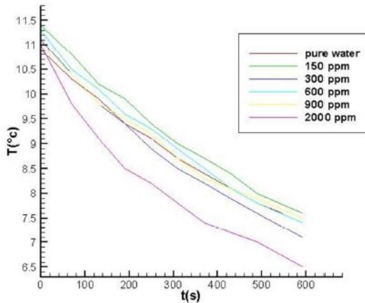
Fig. 8: Evaporator discharging temperature in pure water and different amount of CNT
