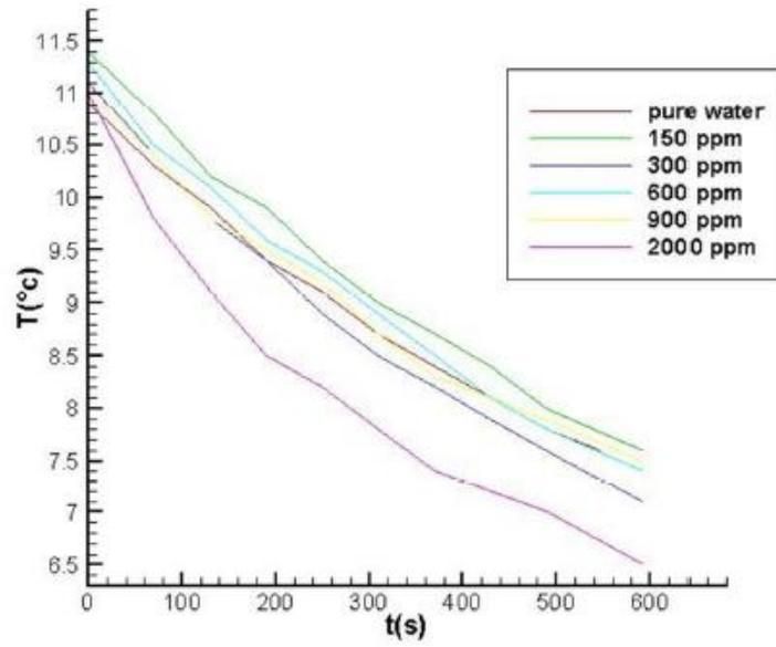
Fig.7: Evaporator discharging temperature in pure water and different amount CNT
