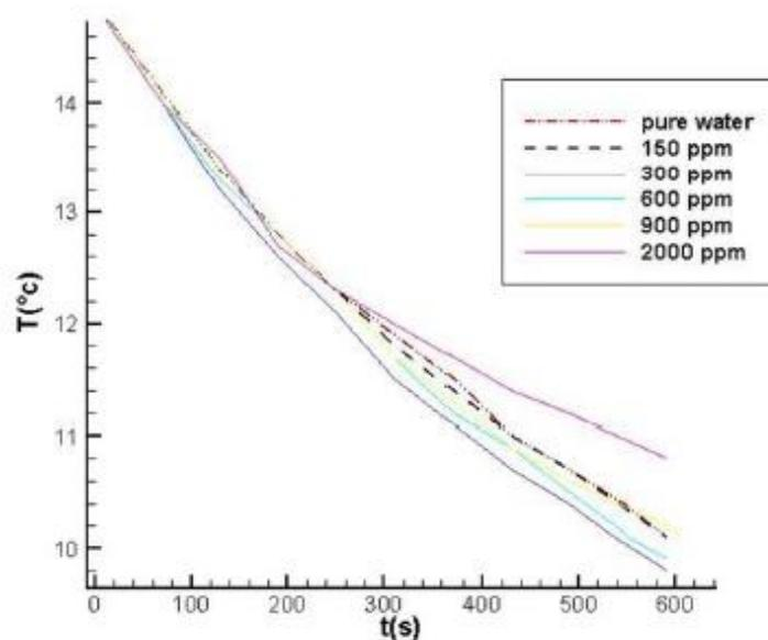
Fig. 6: Evaporator entry temperature in pure water and different amount of CNT
