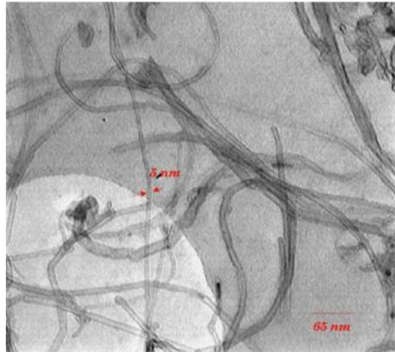
Fig. 4: Typical TEM image of carbon nanotubes.
