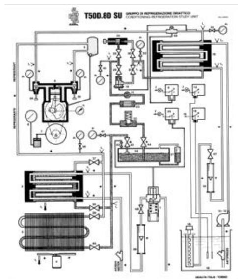
Fig. 5: Schematic of the experimental setup.
