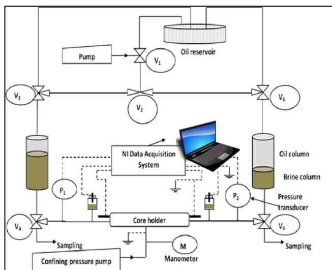
Fig. 3. Experimental set-up for streaming potential measurement [8].
