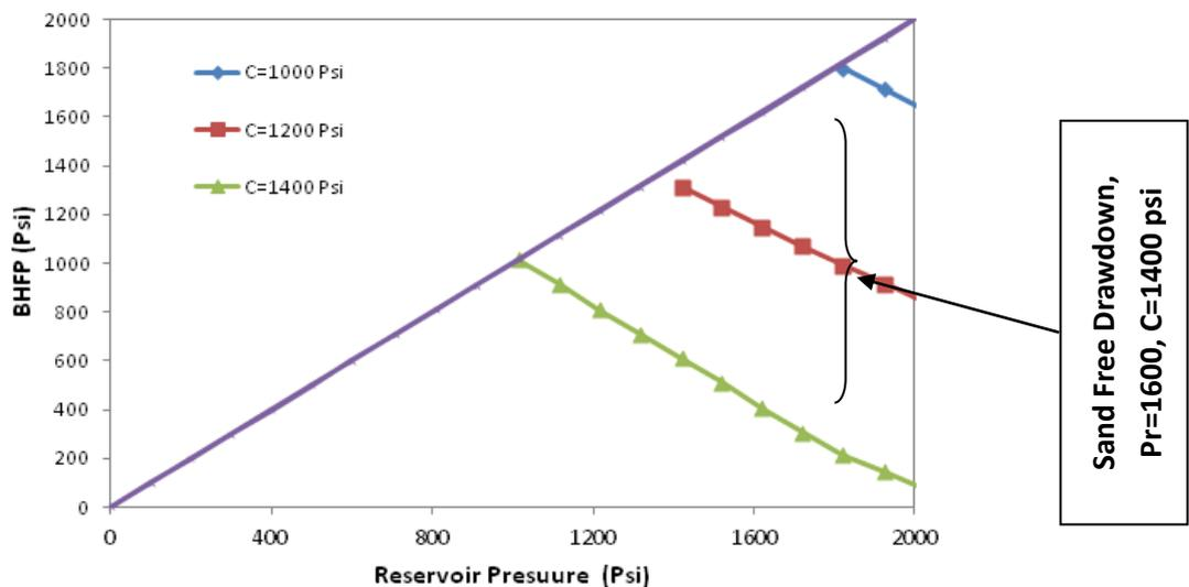
Fig. 6: Sand Free Drawdown Pressure for Three Different Reservoirs Rock Strength
