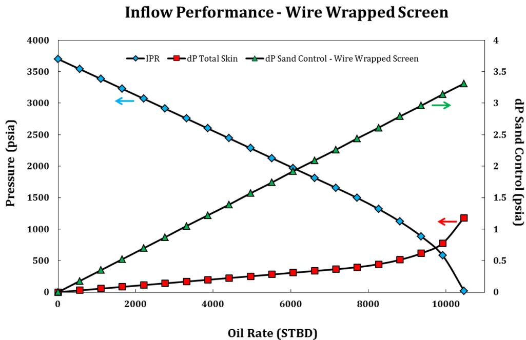
Fig. 10: Inflow Performance Relationship and Pressure Drops in the Case of Wire Wrapped Screen
