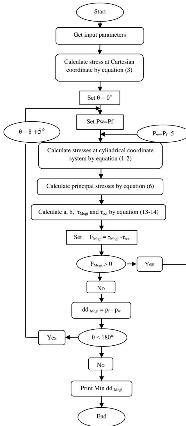
Fig. 1: Sanding Onset Prediction Flowchart According To Mogi-Coulomb Failure Criterion
