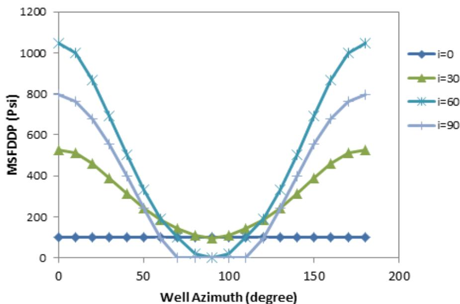
Fig. 4: MSFDD Pressure of the Wells with Different Trajectory in Reverse Stress Regime
