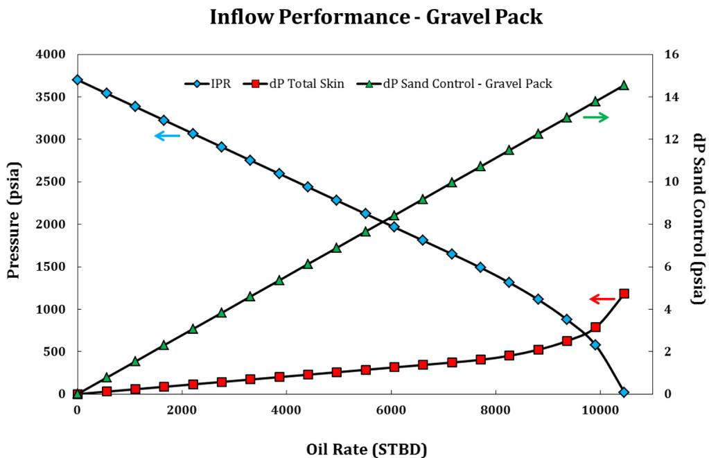
Fig. 7: Inflow Performance Relationship and Pressure Drops in the Case of Gravel Pack
