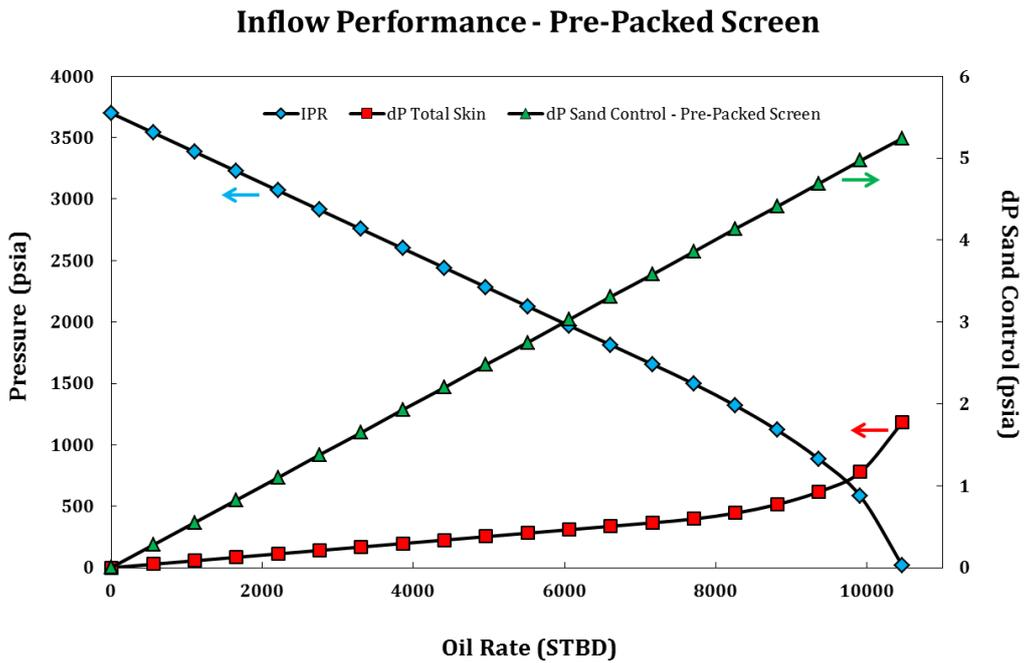
Fig. 8: Inflow Performance Relationship and Pressure Drops in the Case of Pre-Packed Screen
