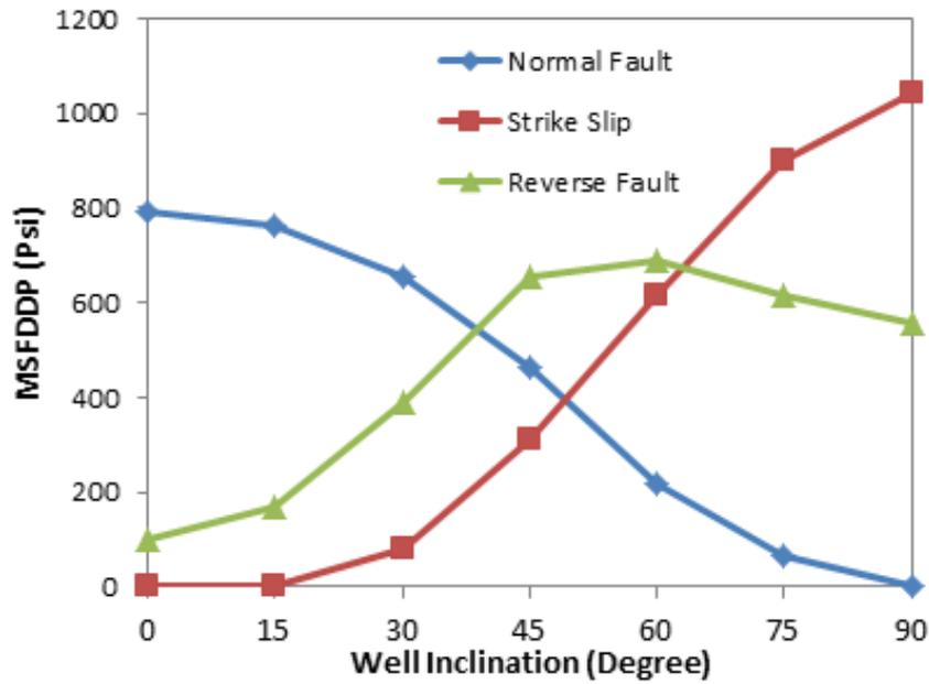
Fig. 5: MSFDD Pressure for Three Different Stress Regimes with Different Well Inclination
