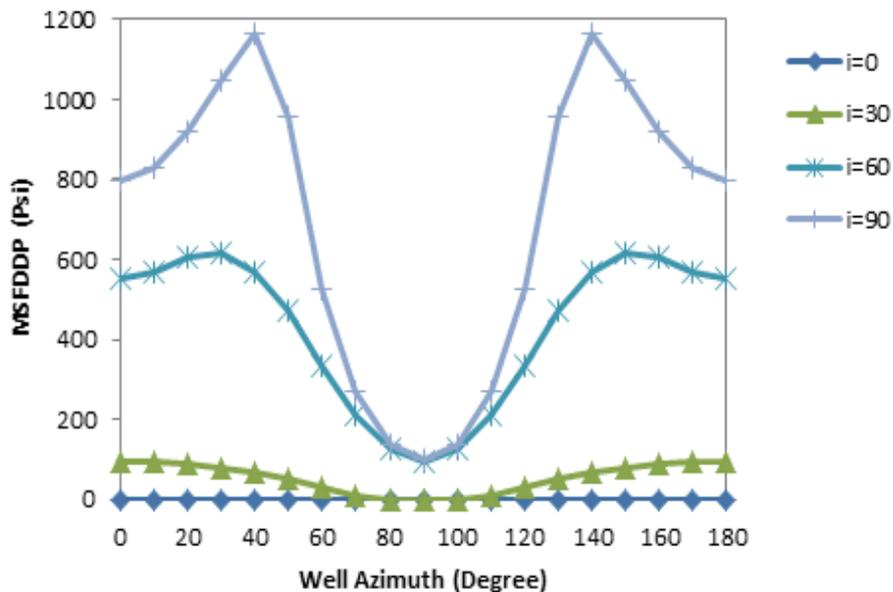
Fig. 3: MSFDD Pressure of the Wells with Different Trajectory in Strike Slip Regime
