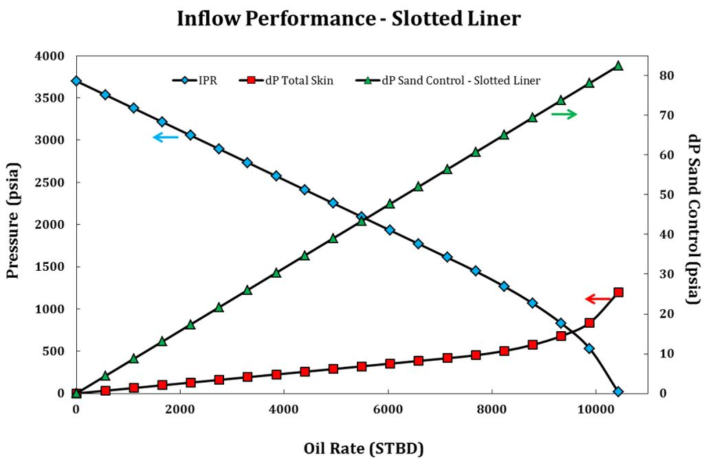
Fig. 9: Inflow Performance Relationship and Pressure Drops in the Case of Slotted Liner
