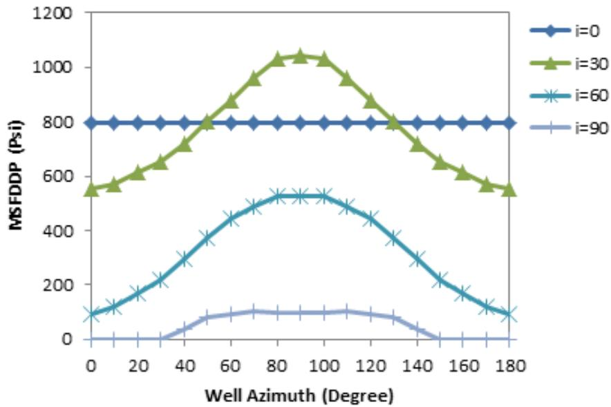
Fig. 2: MSFDD Pressure of Wells with Different Trajectory in Normal Stress Regime
